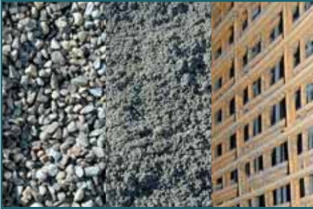
Aggregates, cement and reinforcing steel are the basic raw materials used in reinforced concrete pipe
