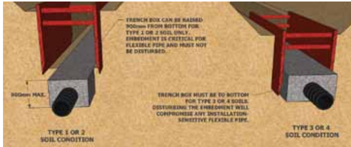
Proper use of a trench box
