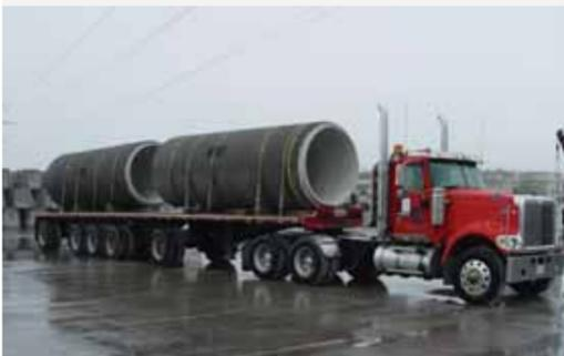
Shipment of 1800 mm (72-inch) pressure pipe leaving plant.
