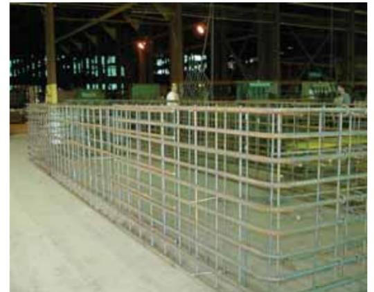
Pre-welded reinforcing assembly for Quick Span mould.
