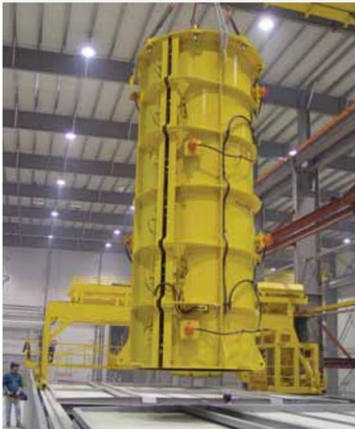
Hydraulically-activated mould jacket elevated over curing chambers.
